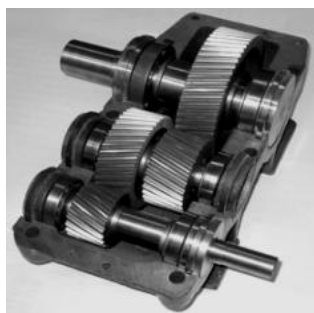
Fig. 5. Double-reduction gearbox with Fig. 6. Stand for transmission ratio inspection noncircular gears
