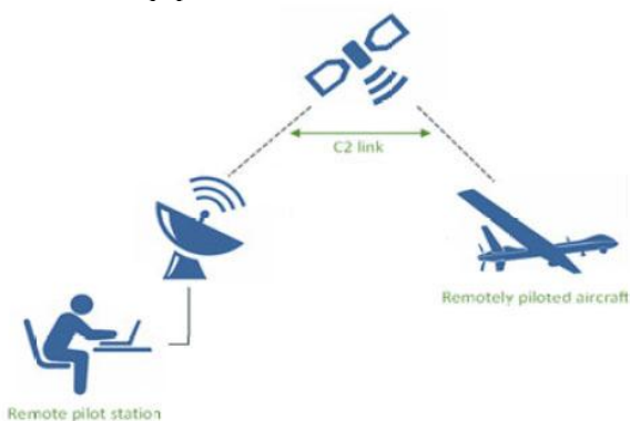
Figure 2. BRLOS Communication Operational Diagram
