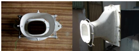
Fig. 3. Experimental model nozzle tips and model axial subsonic ejector
