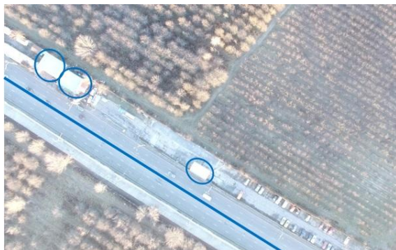
Fig. 1. Different types of landmarks. Linear guidance are marked with blue lines, dot - blue circles.
