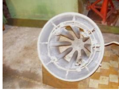
Fig.7. Prototype of ejector with petals at the inlet to mixing chamber
