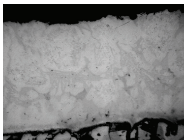
Fig. 3. Structure of melted CEC nickel-eutectic alloy after heat treatment at 1250°C, \times 200
