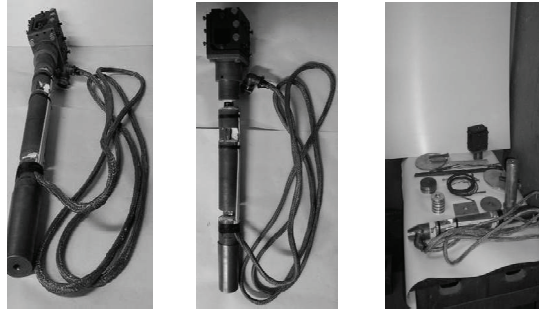
Fig.1 General view of six-component combined strain-gauge balance.
