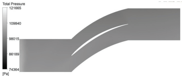
Figure 2 Instantaneous total pressure distribution for the mesh №3 at \lambda = 0.4
