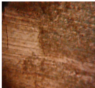
Fig. 3. The topography of steel 45 surface, when the pulsed electrical current of 1 kHz frequency is applied and additional electrode Fe is used
