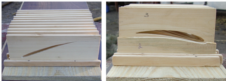
Fig.6. Platform with staples for turbomachine blades row design
