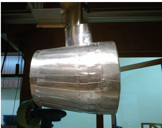
Fig.1 Duct configuration for low airflow velocities.
