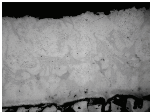
Fig. 3. The structure of remelted CEC after heat treatment at temperature 1250 °C, \times 200
