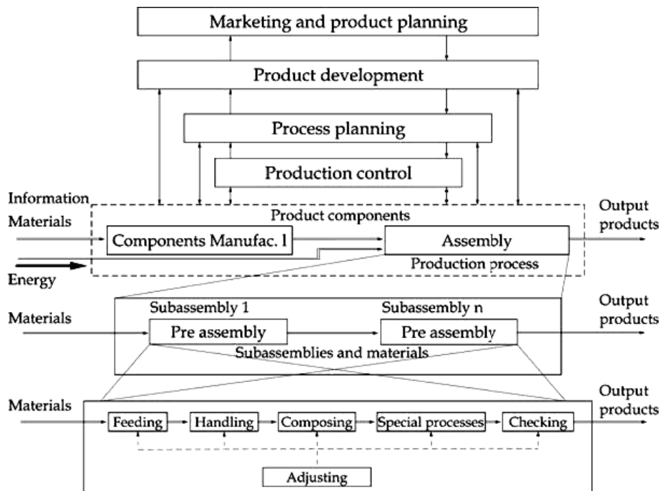
Figure 1. Production process of the computerized robotic vision system
