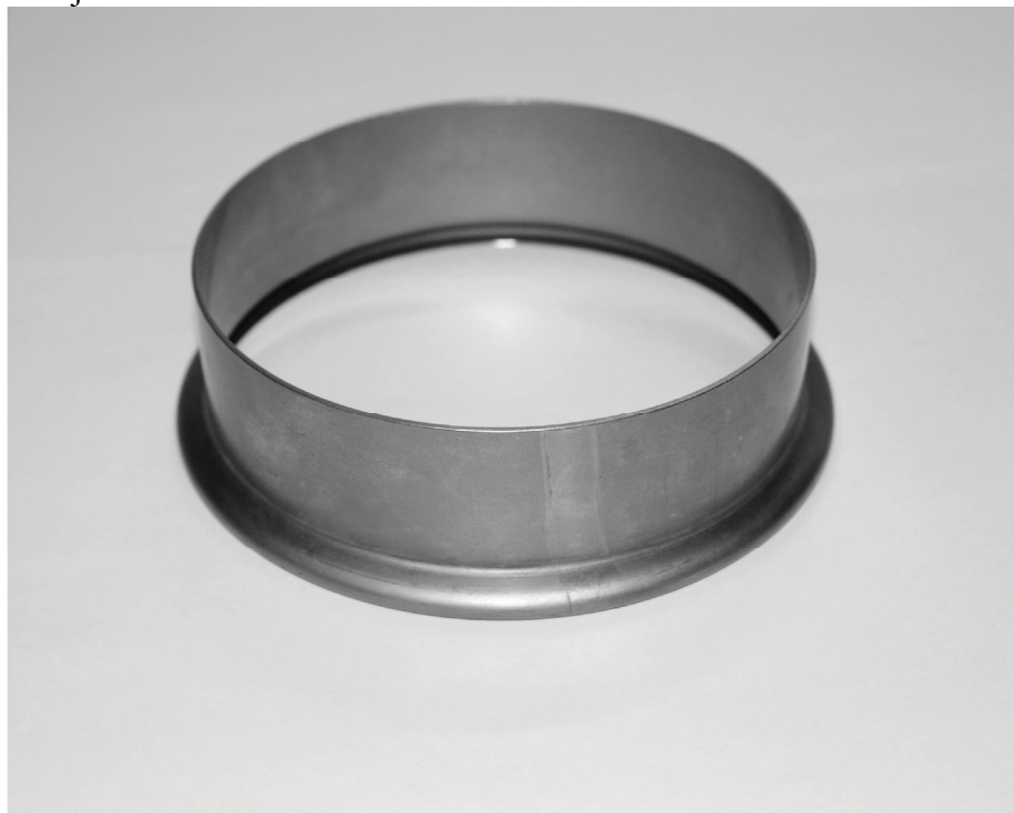
Fig. 1. The lightweight flange of 50 mm in diameter made of titanium alloy PT-7M
