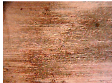
Fig. 4. Friction surface of steel 45, when the pulsed electrical current of 1 kHz frequency and interruption of 6 Hz is applied and additional electrode Fe is used
