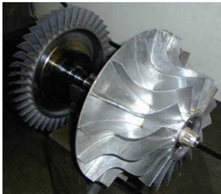
Figure 1. Gas generator of the experimental turbojet engine[1]
