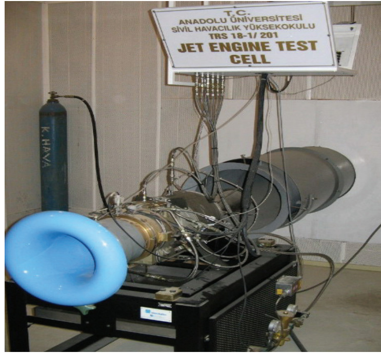
Figure 2. Experimental turbojet engine test cell [4]
