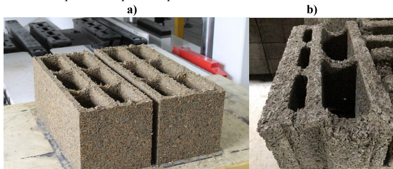
Fig. 1. Types of bioconcrete blocks: a) symmetrical; b) asymmetrical
