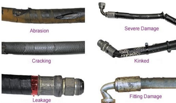
Fig. 2. Examples of Damaged Hydraulic Hose
