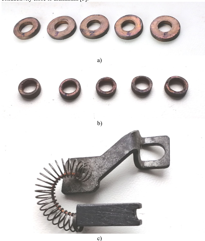
Fig. 4. Experimental testing samples: a) – coated copper samples after testing: b) – uncoated copper samples after testing: c) – graphite brush after testing.
